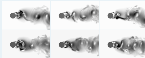
Figure 3: Top: Real-world images. Bottom: Synthesized images by the DCGAN trained on 5,000 LES images over 2,000 epochs with batch size 20.
